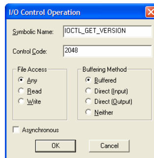
Figure B-4. Dialog box for adding and editing an I/O control operation.
