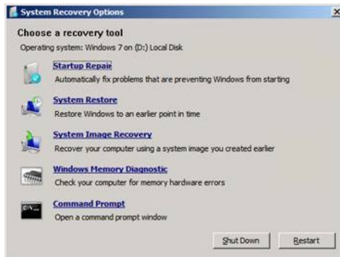
Figure 13-8. The Advanced System Recovery Options dialog box
