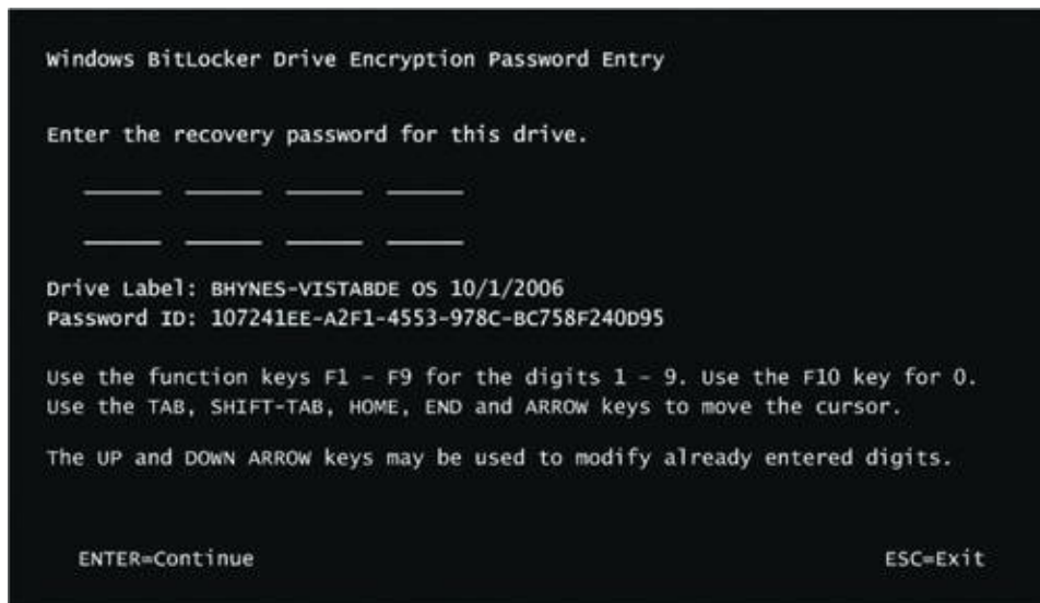
Figure 9-23. BitLocker recovery screen
