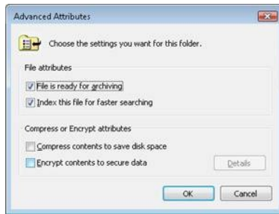
Figure 12-61. Encrypt files by using the Advanced Attributes dialog box
